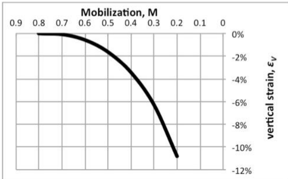
Figure 9 Mobilization, M = K/K_A determines vertical strain due to plasticity.
